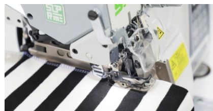
新型独立驱动的上爬齿机构, 专门解决厚料, 多层易滑面料, 易错层面料问题; New independent drive up gear mechanism, specially to solve the thick material, multi-layer easy to slip fabric, easy to split- layer fabric problems;
